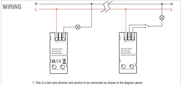
2. You can not connect more than one dimmer in parallel to operate the same charge from two points
